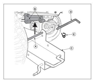
Figure 9. Hitch Latch Pin Installation
